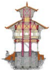
the earthquake - proof steel structure
